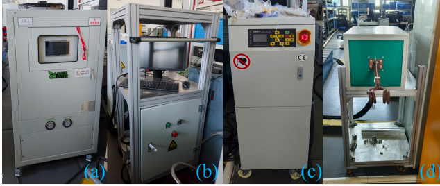
Fig. 3. Induction heating systems: (a) water-cooled chassis; (b) host computer; (c) power control; (d) induction heating coils and transformer.
