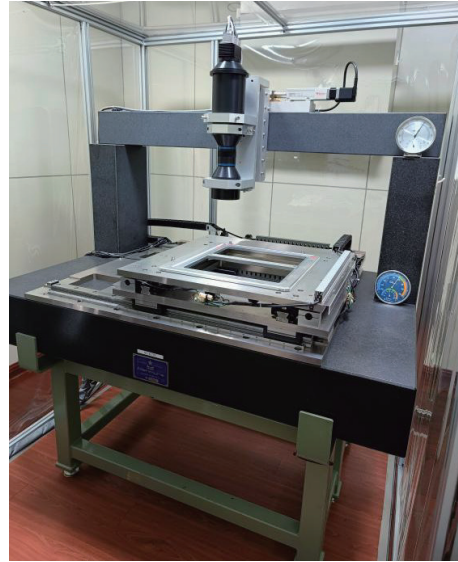
Fig. 1. First high-precision astronomical plate digitizer developed at the Shanghai Astronomical Observatory in collaboration with the Nishimura Co., Ltd. (Japan).
